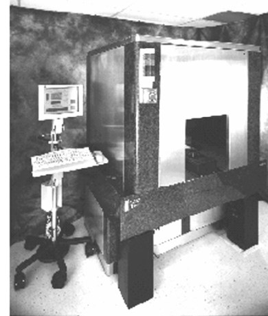
Fig. 14 PC2 automated interference lithography system for patterning 190 nm to 4 micron period patterns
