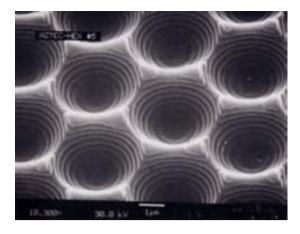
Fig. 3. Aztec honeycomb grating  $(10,300\times)$ .
