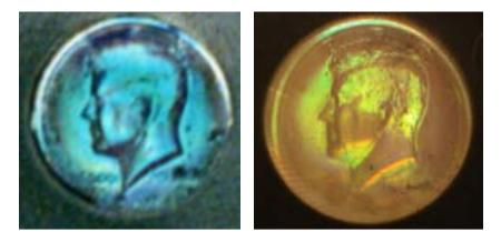
Fig. 6. Aztec single-color holograms. Left image, step height = 121 nm; right image, step height = 182 nm.
