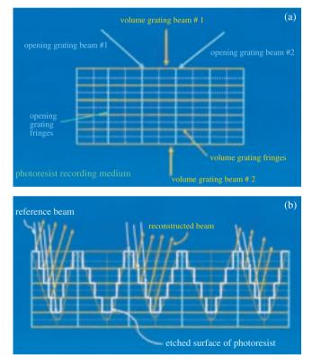
Fig. 2. (a). Construction of Aztec grating. (b) Reconstruction of Aztec grating.
