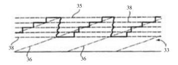
Fig. 5. Aztec asymmetric profile. Photoresist recording medium, 33; top surface, 35; volume fringes, 38; tilted off-axis opening fringes, 36.
