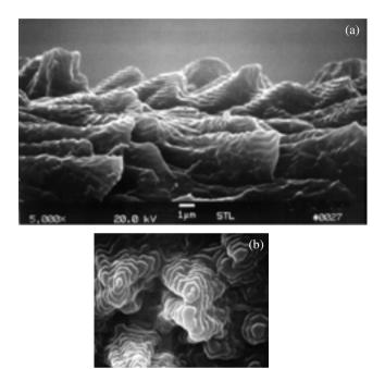
Fig. 7. (a) Asymmetric (blazed) embossed Aztec hologram, side view at  $5000 \times$ . (b) Asymmetric (blazed) embossed Aztec hologram, top view at  $10,000 \times$ .
