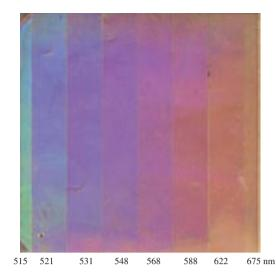
Fig. 4. Aztec colorstripe grating embossed in plastic, showing center wavelengths of each stripe.
