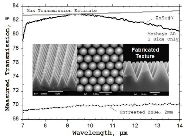
**Figure 1.** Scanning electron microscope (SEM) image of a moth-eye anti-reflective (AR) texture etched in a zinc selenide (ZnSe) window and LWIR transmission spectrum.
