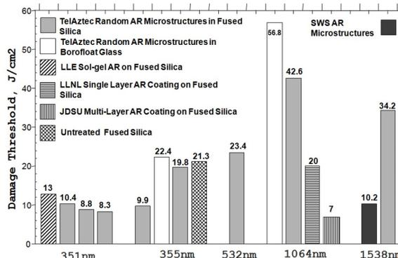
Figure 4. Summary of our LIDT test results compared to results reported elsewhere.<sup>4–8</sup> LLE: Laboratory for Laser Energetics. LLNL: Lawrence Livermore National Laboratory. JDSU: JDS Uniphase Corp.
