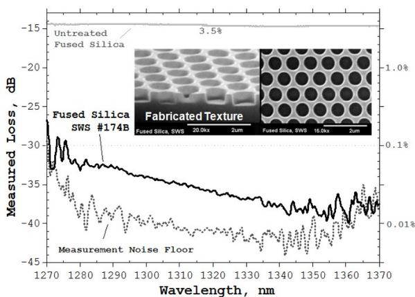
Figure 2. SEM images of a moth-eye, random, subwavelength (SWS) AR texture etched in a fused silica window and NIR reflection spectrum.
