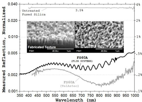
Figure 3. SEM images of a random AR texture etched in a fused silica window and near-UV-VIS-NIR reflection spectrum. FLIR: FLIR Systems Inc.
